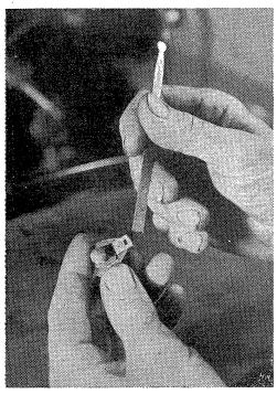
5. Clean and check distributor cap for cracks or corrosion. Corrosion causes current loss, and cracks cause misfiring. Inspect distributor rotor block. If contact is excessively burned, the rotor should be discarded. Otherwise it may be dressed with a point file as shown.
