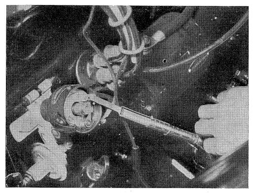
7. Distributor points are designed to operate under a tension of 19 to 23 ounces. The mechanic is testing the spring tension using an SE-1189 Spring Tension Scale. Tension may be increased or decreased as required by bending the point arm slightly. It will be necessary, then, to replace points. Reinstall distributor cap.
