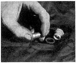
3. Carburetors having a filter element incorporated should have the element removed and cleaned. Remove the fuel pump bowl and clean or replace the screen. If filter element is in fuel pump, it should be cleaned. Clean bowl and reinstall.
