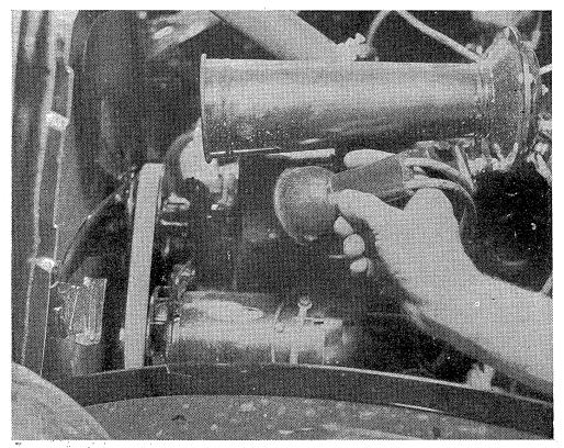
14. Check ignition timing, using a synchroscope or timing light. An instrument similar to that shown is available under SE-939. A chalk mark on the crankshaft pulley notch will facilitate the synchronization operation. Engine speed should be at approximately 350 r.p.m.
