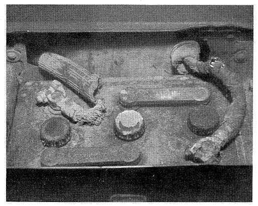
13. Check battery cable connections and the condition of the cables themselves. Worn or frayed cables and connections as shown must be replaced for they affect a material current loss. The battery ground connection must be clean and tight. A poorly grounded terminal will cause hard starting and poor operation. Sulphated terminals can be easily cleaned with common soda and water.
