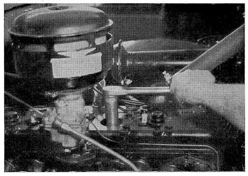
10. Reinstall spark plugs using new gaskets. Use a properly fitting socket wrench for an ill-fitting socket as an end-wrench may slip and damage the porcelains. Do not exert excess pressure in tightening plugs. Only sufficient pressure to compress the gasket is required. Connect spark plug wires.
