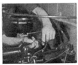
Check the high tension (spark plug) wires for faulty insulation and for faulty terminals. Faulty insulation will appear brittle and will crack easily when wrapped around the finger. Test as shown and replace wires if cracks appear, for otherwise
