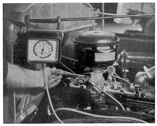
15. Adjust carburetor idle speed to approximately 350 r.p.m. A vacuum gauge similar to the SE-1199 Vacuum Gauge shown should be attached to intake manifold and used, unless a combustion tester (exhaust gas analyzer) is available.
