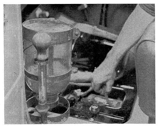
12. Water level should be corrected to 3/8" above the separator plates. Add only distilled water. The water filler bottle shown is the SE-617 Battery Water Filler. Reinstall vent caps after ascertaining that the vent holes are open. CAUTION—Keep open flames away from storage batteries.
