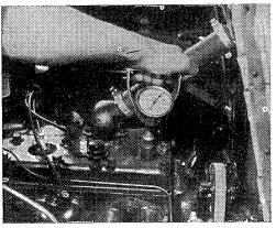
A tune-up will be of little value if the 1. A tune-up win be of asset in valves are in poor condition resulting in the cyllow and unequal compression in the cylinders. A compression test should be made to establish that compressions of the cylinders are equal to within ten pounds of each other. The mechanic is shown using a Compression Tester SE-834.
