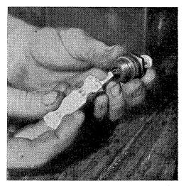
9. Regap spark plugs to .028" to .032" using a round-wire gap gauge. The gauge in use in the illustration is the SE-1152 Spark Plug Gap Gauge. Each mechanic should include a similar one in his tool kit. Flat gauges are inaccurate and impractical.
