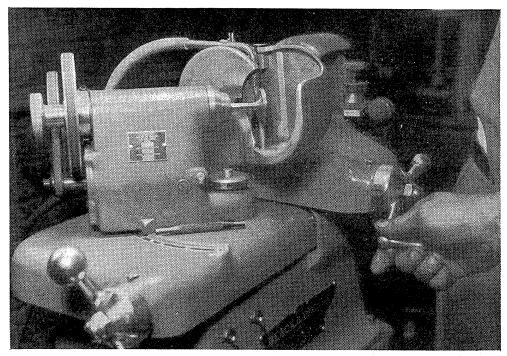
7. After the valves have been thoroughly cleaned they are ready for refacing. Here again precision equipment is necessary so that the valve faces are ground true and smooth, maintaining the proper angle. The equipment shown is a modern wet type grinder.
