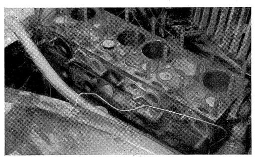
3. Electrical connections, cylinder head and manifolds are now removed preparatory to subsequent operations.
