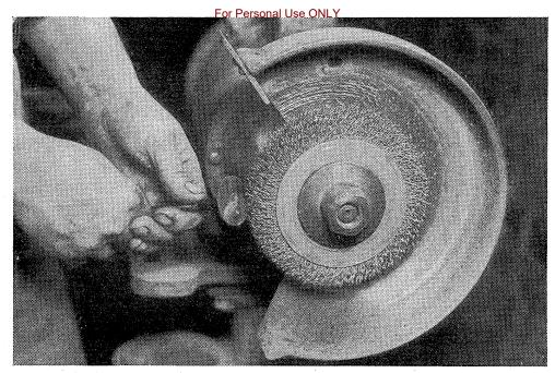
5. After the valves have been removed from the block they should be carefully cleaned and inspected. A power-operated wire brush is best adapted to this purpose, for such a brush is both rapid and efficient. Any valve which is badly burned should be discarded without further attention.
