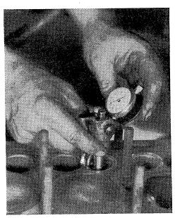
11. After the seats have been properly ground, as shown in Illustration 10, they should be checked with an accurate dial indicator mounted on the same arbor or pilot used for the grinding operation. When valve-face and valve-seat angles are identical it is possible to hold maximum runout within .002".
