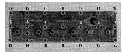
15. (Left): The nuts should be drawn down a little at a time in the sequence shown until the specified tension of 60-foot pounds h as been attained.
