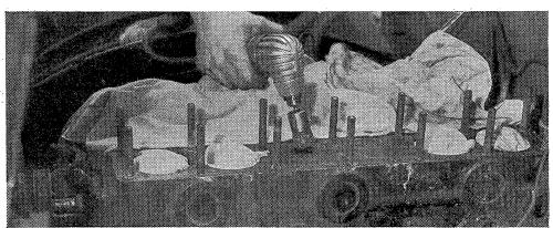
6. Accumulated carbon must be removed from the top of the block, the tops of the pistons, and from the combustion chambers in the cylinder head. Clean cloths placed in adjoining cylinders and parts will prevent carbon and abrasive from being scraped into them. A scraper or wire brush will be found best for carbon removal, and compressed air may be used after the operation for removing the loosened carbon.
