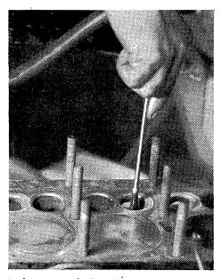
6. An accumulation of carbon is generally found deposited in the valve stem guides. Suitable tools should be used to clean the guides before proceeding with the work. The illustration shows S.E.-7701 valve guide cleaner in use.
