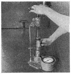
13. Valve springs should be carefully checked for tension before installation. The recommended spring tension when compressed to  $1^{15}_{16}$  inches is 83 to 88 pounds.
