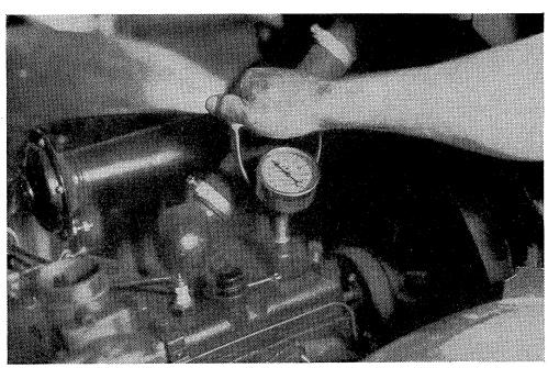
1. A compression test on each cylinder will substantiate the necessity for valve reconditioning. Such tests should be made with compression gauge S.E.-834 or its equivalent. A variation in compression between cylinders of 10 or more pounds is cause for alarm.
