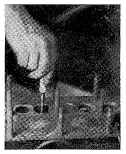
**9.** After valve guides have been cleaned they may be checked for wear with a Go and NoGo gauge, such as S.E.-145 shown in this illustration. If guides are worn excessively they should be replaced. Recommended valve stem clearance in the guides is:
