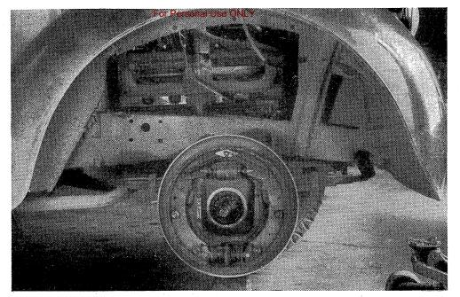
2. Drain radiator, remove hood, remove right front wheel, and right front fender apron, and support truck on steady-rest. Removal of these parts permits easier access to the engine.
