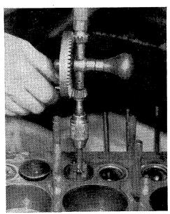
12. When the seats in the block have been ground to the desired width and location, a good check of accuracy of the combined valve refacing and block reseating operation is to lap the valves lightly to their seats, using a fine grade of compound. This serves merely as a test, for lapping of valves must not be considered a substitute for a grinding operation. A poor grinding job cannot be corrected by lapping. This picture shows a common type of tool used for the lapping operation.
